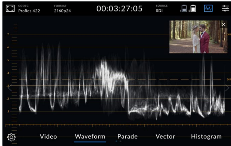
Tapping the preview icon will display the scopes full screen with the video image in the top right corner of the screen
